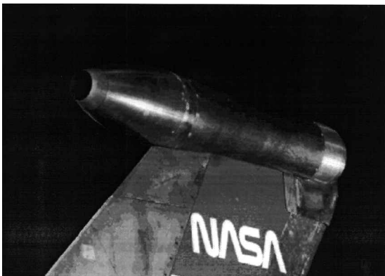
Fig. 2 Photograph of the model in the 40 × 80 ft wind tunnel.
